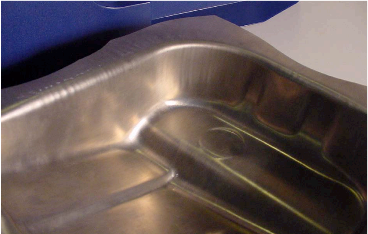
Figure 7-14 Wrinkles in the aluminium pedal box
